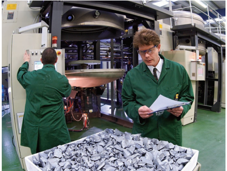
Quartz crucible containing polysilicon feedstock before loading into a crystal-growing furnace. Today, demand for silicon in the photovoltaics industry is greater than for the microelectronics industry.
